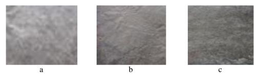
**Fig. 1** Physical appearance of the products after electrospinning. (a) control- PLA alone (b) extract from *C. globosum* and (c) extract from *C. cupreum*
